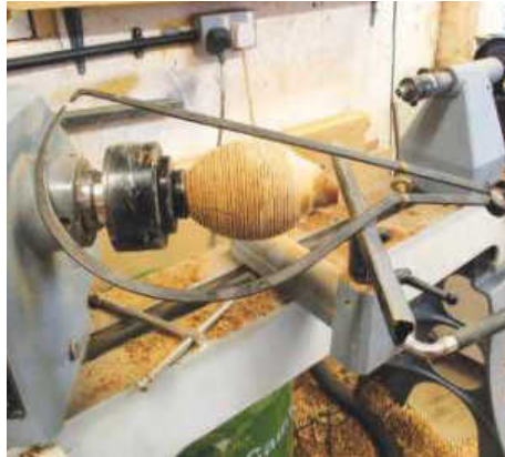
STEP 21. Measuring the wall thickness will require some specialist callipers once you go past finger depth. The spring-loaded ones from Veritas are fantastic, albeit expensive
